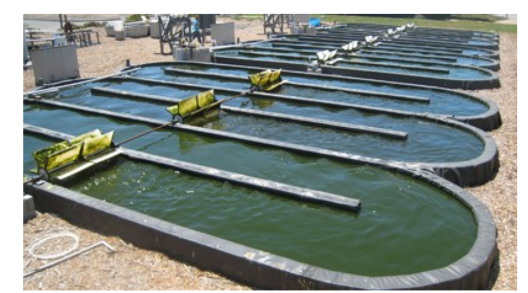
Fig. 2: Example of Open Algae Pond for Cultivation
