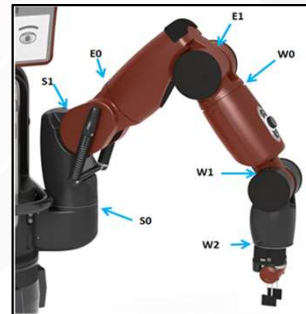
Seven Rotational Joints of Baxter
